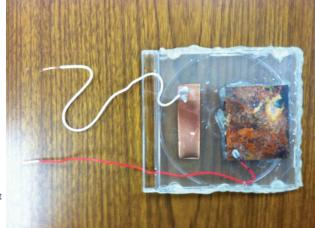
Step 8: Create a small hole for each wire in the CD case so that the non-connected end of the wire can be fed through to connect with the voltmeter on the outside. Make sure the holes are toward the hinge end of the CD case. A pair of scissors can be used to take out a small piece of plastic for this.
