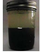
7. Put the jar on a table and let the soil settle out for 40 seconds, mark the level of soil on the jar. This is sand portion in the soil.
